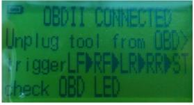
When you see any of the screens above, unplug the Sensor-Aid from the OBD II cable and in the same MMY in the Sensor-Aid, go out of the OBD II function and select the Diagnose function. Please trigger each of the sensors individually in the sequence shown previously.
