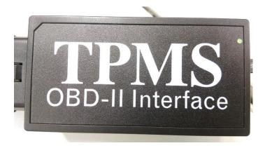
If the OBD II module displays a continuous red light, it indicates that the ID writing failed and you should turn off the car's ACC, disconnect the OBD II Module, plug it back and then turn on the ACC before a new attempt.
